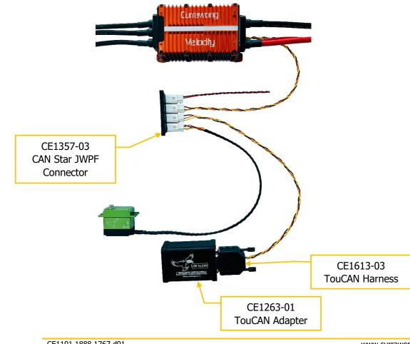
The TouCAN is a fully electrically isolated USB to CAN adapter for the integration and testing of in-situ CAN devices. The TouCAN provides advanced protection against ground shift and electrical noise, ensuring the safety of the host PC. It also provides optional bus termination for user convenience. Currawong offers a matching harness for the TouCAN.
